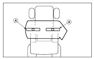
5. Turn left blade parallel to tractor axle. Hold drive belt and turn right blade parallel to axle.
